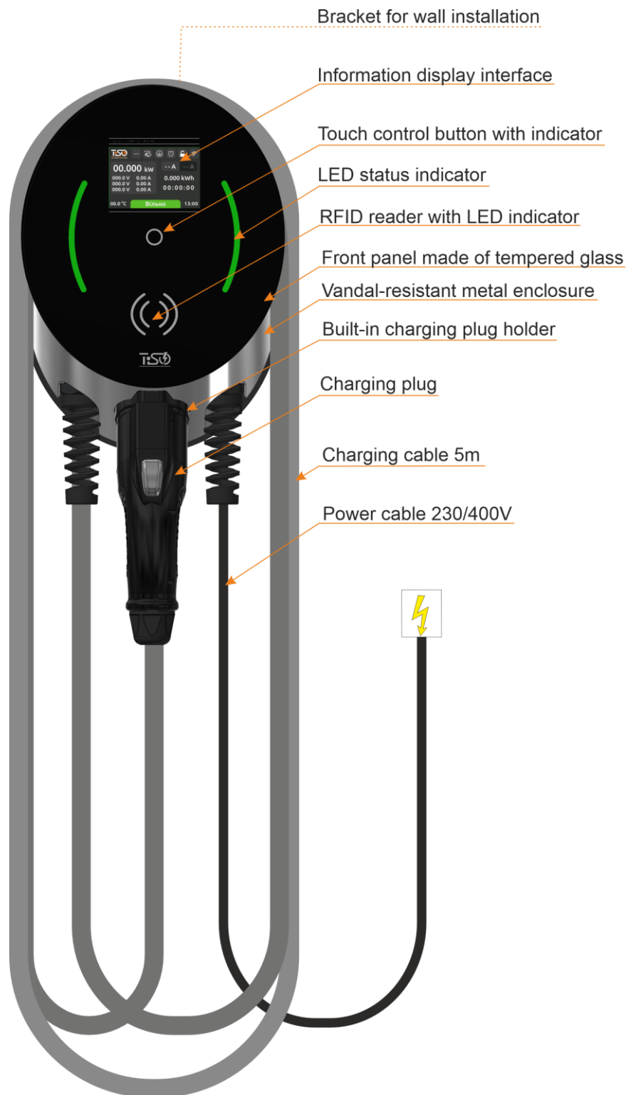
Fig.1 – General view of the station
