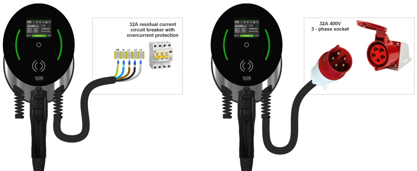
Fig. 7 - Three-phase charging station connection options
