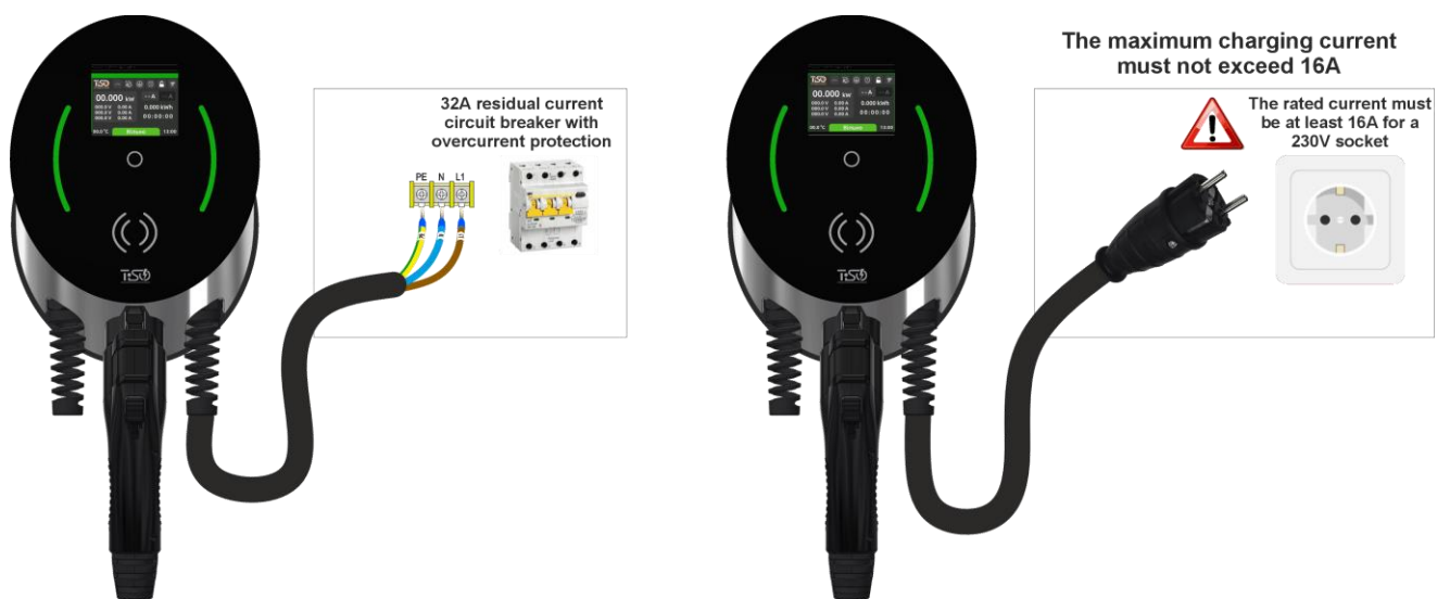
Fig. 6 - Single-phase charging station connection options
